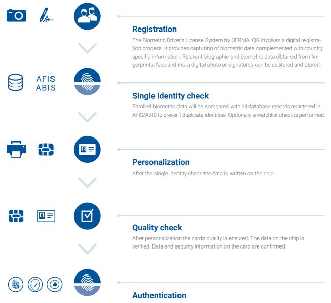
Live Fingerprint/Iris/Face comparison with the data stored on the chip. (On-card matching and off-card matching).
